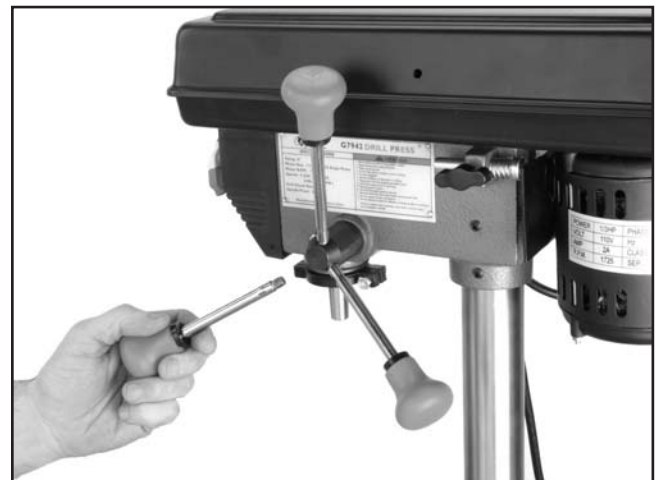
Figure 12. Installing feed handle.
